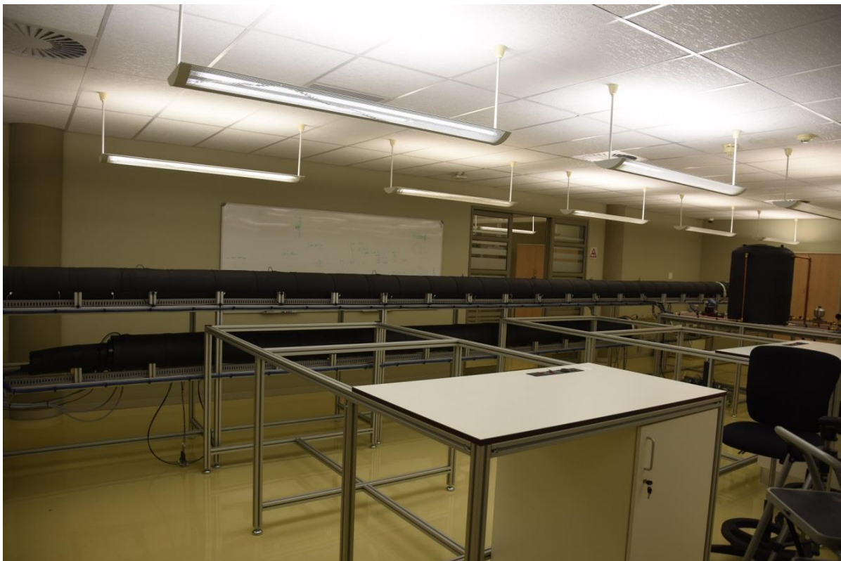
Figure A.5: Photo showing the full length of the insulated test section (bottom shelf). The table in the centre of this photo is exactly the same as the table in Figure A.1, thus everything added to the table in Figure A.1 was done by the Author and 2 fellow students in the time frame of 8 months.
