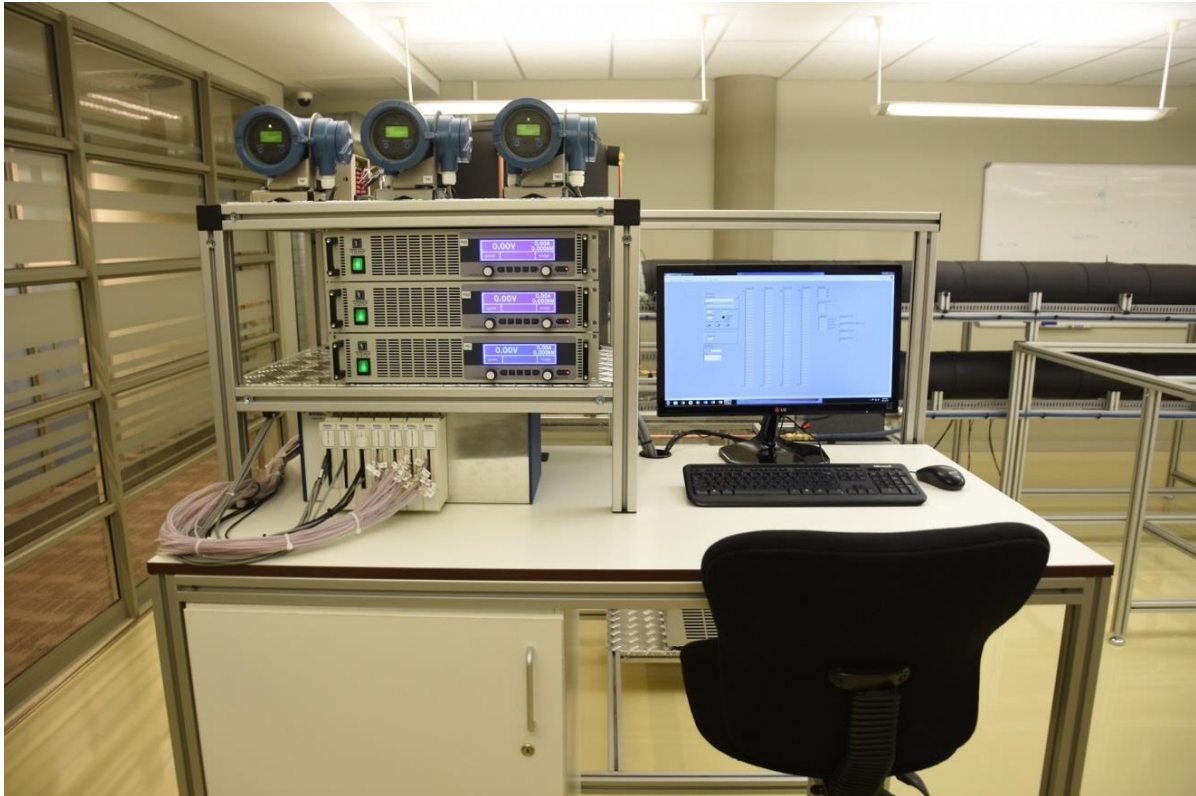
Figure A.4: Photo showing the flow meter displays, power supplies, data acquisition system and computer.
